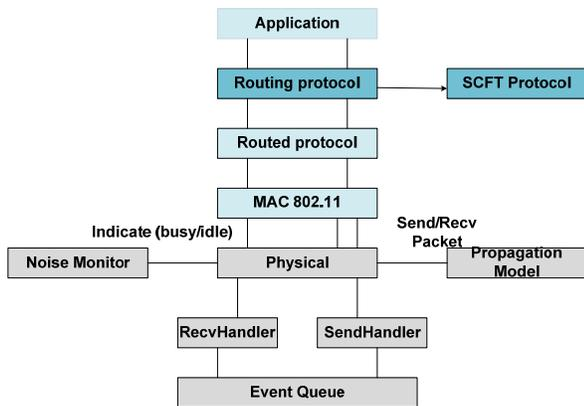
Fig. 1. The architecture of a VANET system using the proposed routing protocol.
