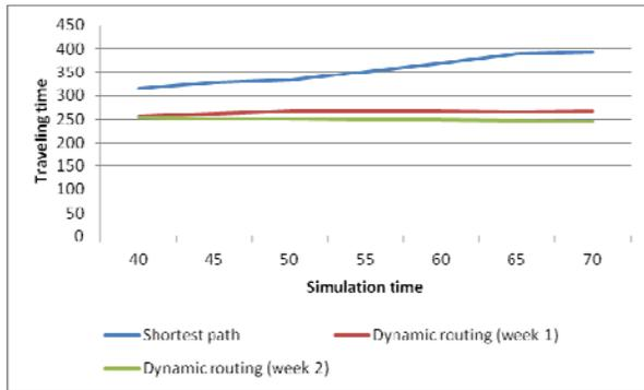
Figure 7. The average traveling time: adaptive traffic lights, 500 cars / hour / lane.
