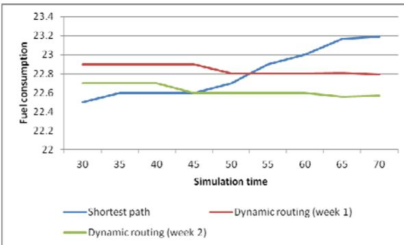
Figure 8. The average fuel consumption: adaptive traffic lights, 500 cars / hour / lane.
