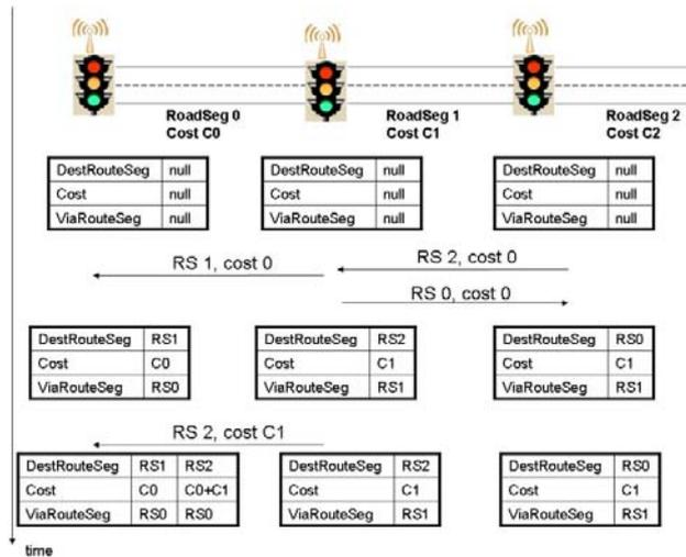
Figure 3. The distance-vector routing approach for route exchanges.
