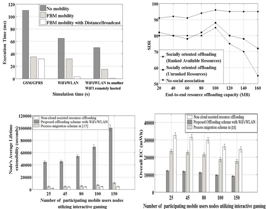
**Fig. 3 (a)-(d).** Comparative evaluations and results obtained for the social offloading regarding the (a) Execution time through simulation; (b) Successful delivery rate with the End-to-End resource offloading capacity based on the “friendship” model; (c) Average node’s lifetime extensibility with the number of mobile devices for three different schemes in the evaluated
