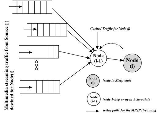
Fig. 2: A schematic diagram of the caching mechanism addressed in this work
