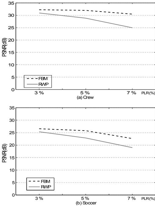
Fig. 4: Average PSNR for three loss connectivity scenarios
