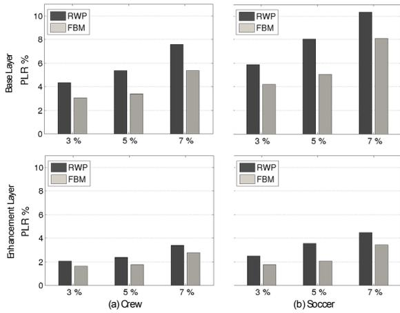
Fig. 3: Average Base and Enhancement Packet Loss rate for three loss connectivity scenarios
